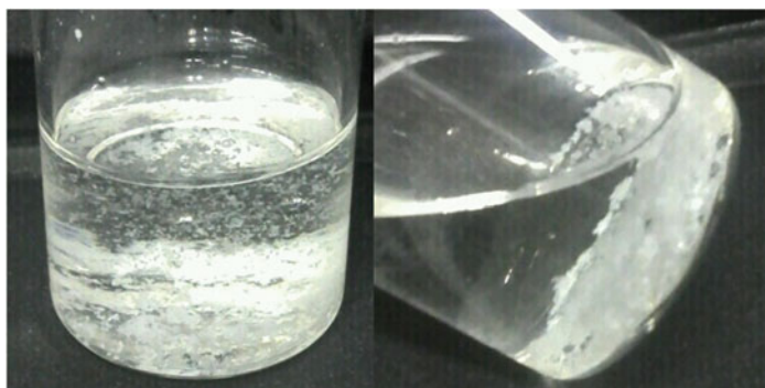
Figure 4. Image of PS-MeOH and PS-EtOH solutions prepared by mixing the PS-powder and alcohols, such as methanol and ethanol.
